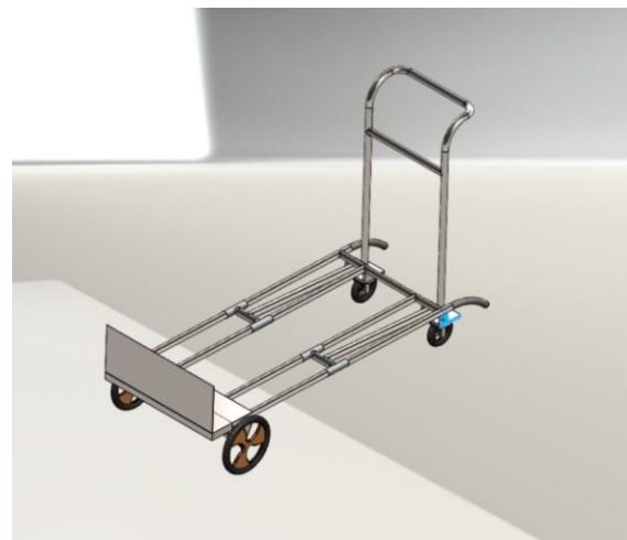
Figure 1. CAD view of the horizontal trolley configuration.
