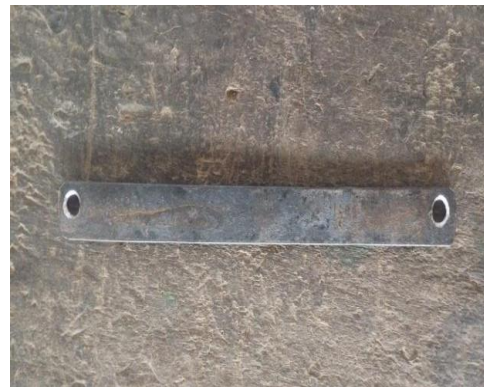
Fig. 8. Connecting rod (flat mild-steel bar).
