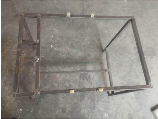
Fig. 5. Fabricated mild-steel frame with castor wheels.
