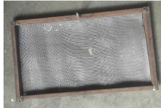
Fig. 10. Final sieve-net assembly ready for installation.
