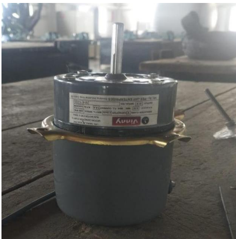
Fig. 6. DC motor (Vinny Electric, 1/5 HP, 1600 RPM).
