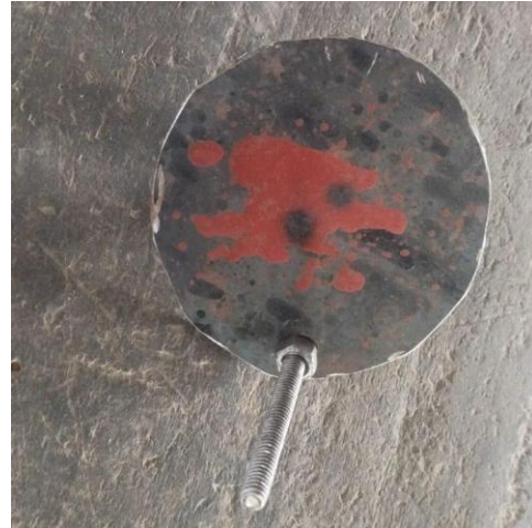
Fig. 7. Crank disc with offset threaded stud.
