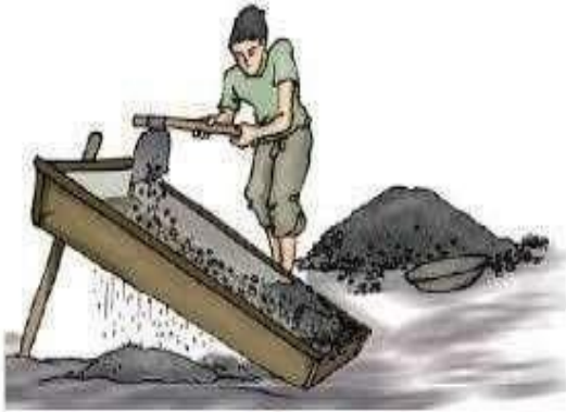
Fig. 1. Conventional manual sieving method.
