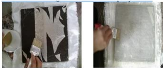
Figure 4 depicts the process of attaching the Glass Fabric to the Core.
